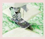
The long guide at the center of the presser foot fits perfectly in the seam line to stabilize stitching.
