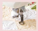
With the feed dogs lowered, you can freely move the fabric to draw using stitching.
