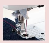
Press the black button to keep the presser foot horizontal in order to smoothly begin sewing at a thick seam.
