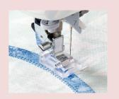
Since the front and back of this presser foot are short and transparent, appliqués and designs are easy to see, and you can easily sew sharp curves. The pin at the back keeps the presser foot horizontal, stabilizing it even when sewing appliqués.
