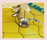
With a distance of 1/4" (6.5 mm) from the needle entry point to the outer edge of the presser foot, sew using a ruler as a guide. The front of the presser foot is lowered, making it easier to see the needle area.
