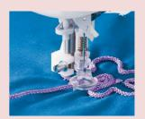
This presser foot has a hole for supplying cording to be sewn over. With the feed dog lowered, you can freely move the fabric to create simple embroidery with cording.
