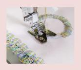
This foot has a claw at its center. It is used for forming loops by laying the thread over the claw. This presser foot can be used for sewing decorative stitches on workpieces by making three-dimensional thread loops and fringes on the edge of the fabric with your favorite threads.
