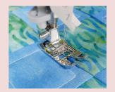
This presser foot has a shorter guide at its center. With this shorter guide, smoother feed of the material is promised. Furthermore, it is expected to reduce uneven material feed. The marks on the left side of the presser foot will be the guide for the outline quilting. By changing the needle base line, you can sew the single lap stitching with ease.
