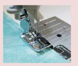
Always ensure needle is set to center straight stitch. Align the edge of the fabric with the presser foot guide to easily sew with a seam allowance of 7 mm. Since the needle drops into a small round opening, the seam is stabilized to create a perfect straight stitch.
