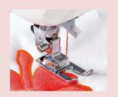
The wide opening at the front of this presser foot makes appliqués and designs easy to see, which is useful for curvy decorative stitching. The groove along the bottom of this presser foot ensures that the presser foot does not catch on the stitching, so the fabric will be smoothly fed.
